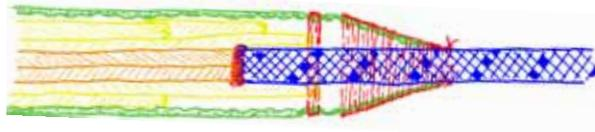
5 Trim the rest of the core bundles to give a gradual taper over a length of 15 cm.
