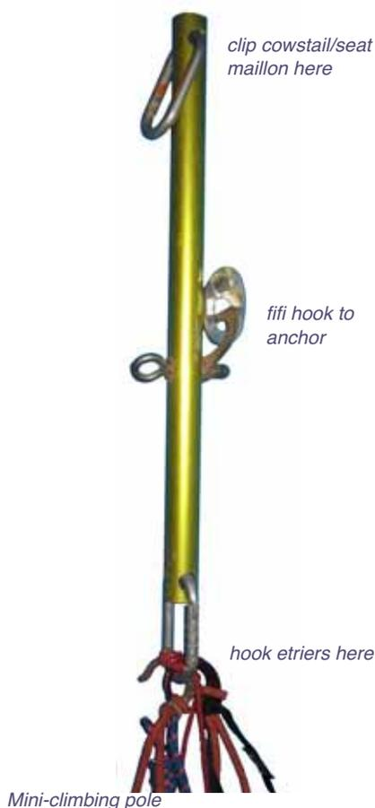
A mini-climbing pole as sold by Raumer (*Allonge Stick-up*) is an 80 cm length of aluminium tube with attachment holes at the top and bottom and a hole about 1/3 of the way along.
