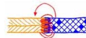
4 Reinforce the fused joint with stitching.
