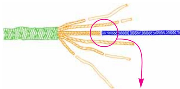
The rope must taper smoothly from 8 mm down to a 3 mm diameter, 30 cm long tail.
