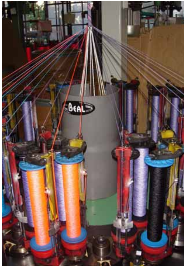
Kernmantle rope under construction (Beal factory/website)
