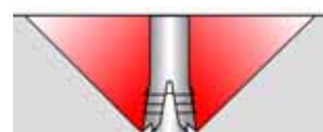
The stressed zone around a bolt has a radius at least as big as the anchor length
