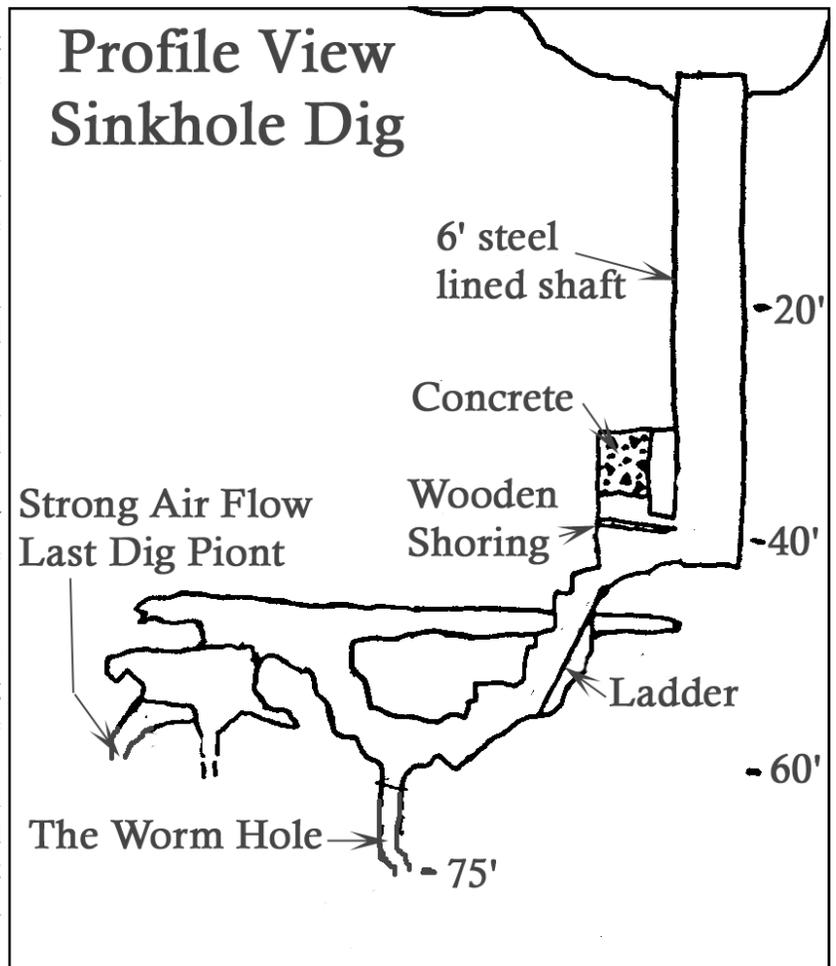
The first shoring to go in to the dig was an 11-foot long section of the 6-foot diameter 5/16-inch wall pipe. This section weighed about 2700 lb.
