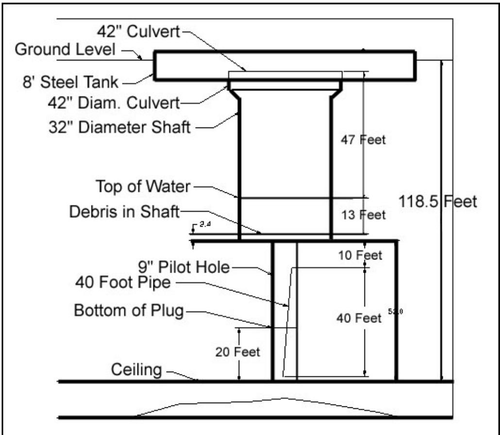
T-Junction Dig Cross Section Vertical scale reduced by a factor 12
