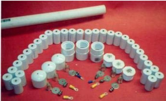
Time to build. First thing I did was drill a hole in each cap. Then solder a washer on the wide part of the spring. Next slide the bolt through the washer into the hole in the PVC cap, but do it from the inside. Next put a ring terminal on the bolt then the nut. Put a screwdriver through the spring and a wrench on the other side and tighten.
