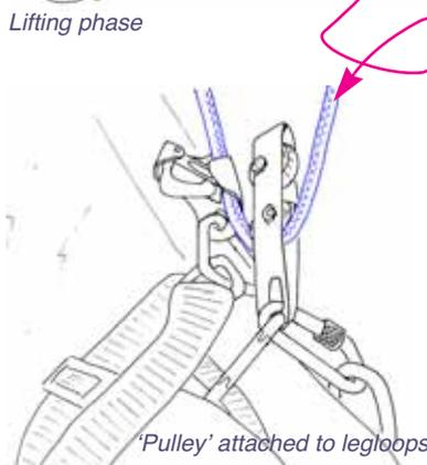
'Pulley' attached to legloops
