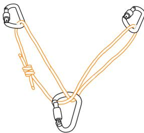
Use rope, never tape. Twist the loops so that if any one anchor fails, the belay doesn't undo.
