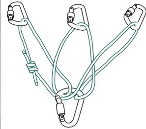
Load distributing anchors —use 3 normal anchors, or 2 very good ones.
