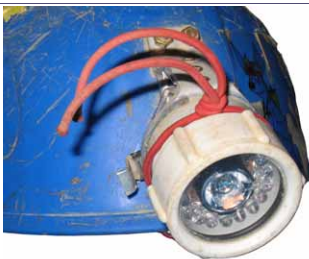
One of many prototypes. A single central 'Luxeon' for spotting surrounded by 18 x 5 mm LEDs for normal use. Each set of LEDs is separately powered and switched to provide redundancy
