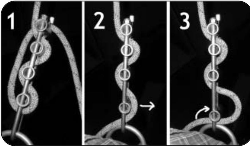
1. Micro-rack rigged with all bars including the hyper-bar.
