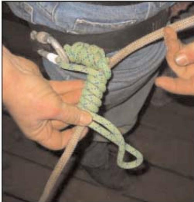
rappel stops. If you freak and let go of the rope with your brake hand, or are injured, knocked out, or whatever, and LET GO of the French Wrap, it will set, putting tension on the rope and rack, stop-ping the rappel! Either way... you stop the rappel and do not fall to your death.
