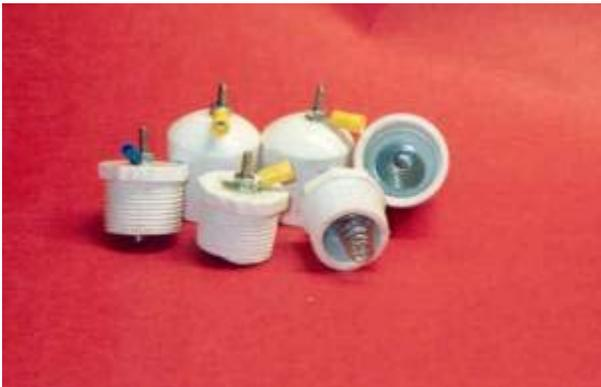
Once you have all six plug ends done then glue the three cap sockets and the three female adapters to the PVC pipe.
