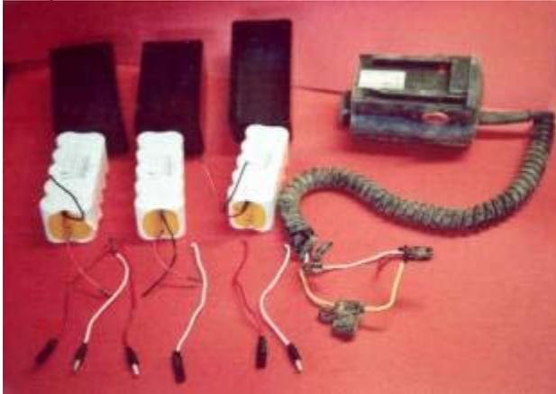
So I ordered three 12-volt 3Ah presoldered battery packs from [www.batteryspace.com](http://www.batteryspace.com). I order the presoldered because if you solder a charged battery you take a chance of destroying it. Some have actually exploded. With the batteries soldered together you won't lose as much electricity
