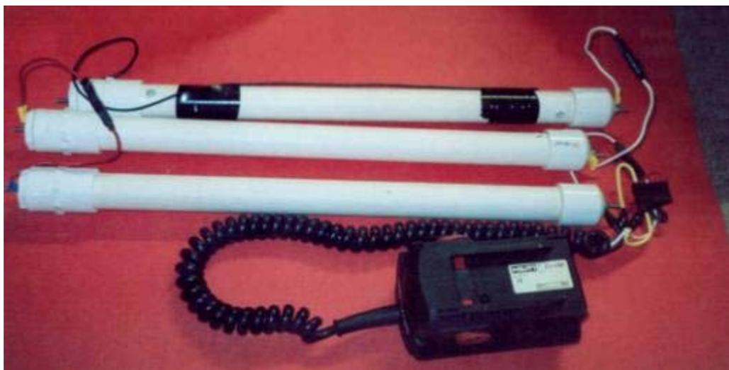
First thing is to go shopping. I bought 30 3000-mAh batteries off [Www.batteryspace.com](http://Www.batteryspace.com) and three smart chargers. Then I went to the local hardware and got PVC pipes and fittings, and the local auto parts store.
